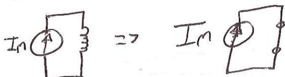
A steady state circuit w/ DC source, inductor acts like a short circuit
