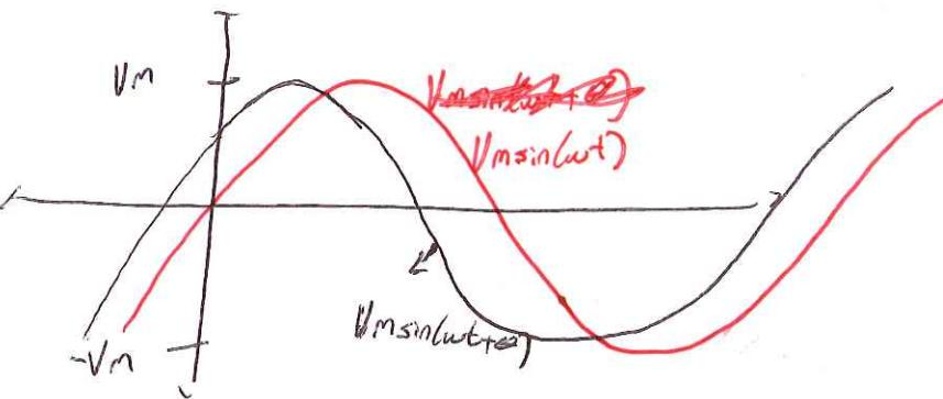
$V_m \sin(\omega t)$  lags  $V_m \sin(\omega t + \theta)$  by  $\theta$  rads
