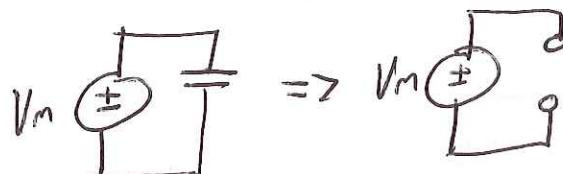
A steady state circuit w/ DC source, capacitor acts like open circuit.
