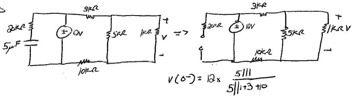
$$V_{c(0-)} = 12V = V_{c(0+)}$$
